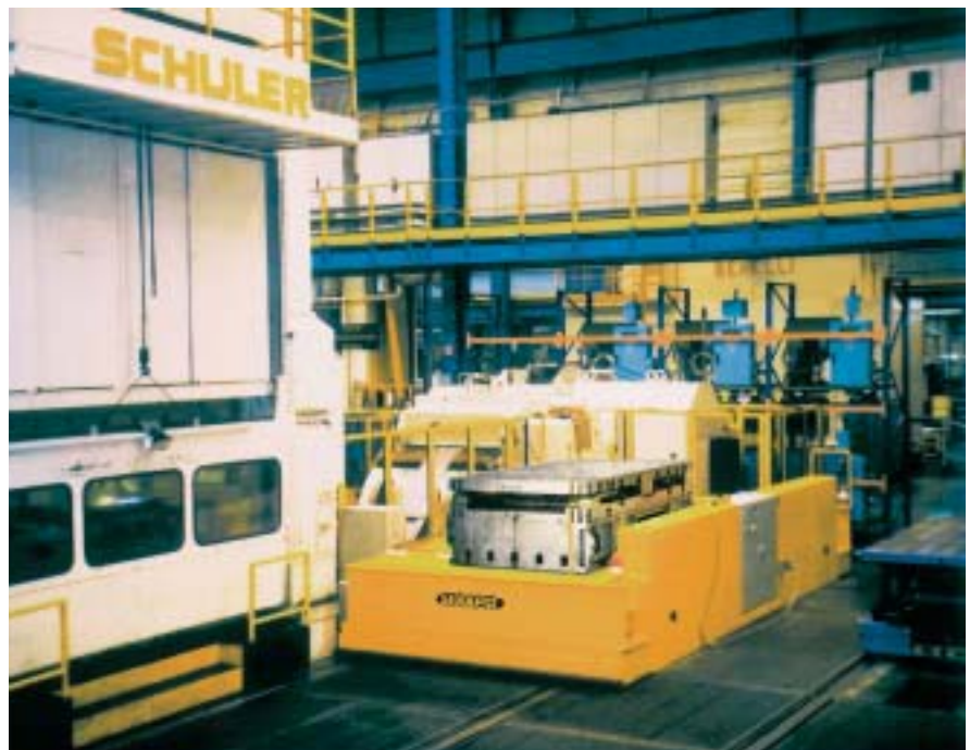
Traditional manual die-changing methods often require multiple employees and hours of downtime. This automatic two-position die cart is one part of an effective quick-die-change system that may reduce die exchange to one employee and as little as 5 min.
