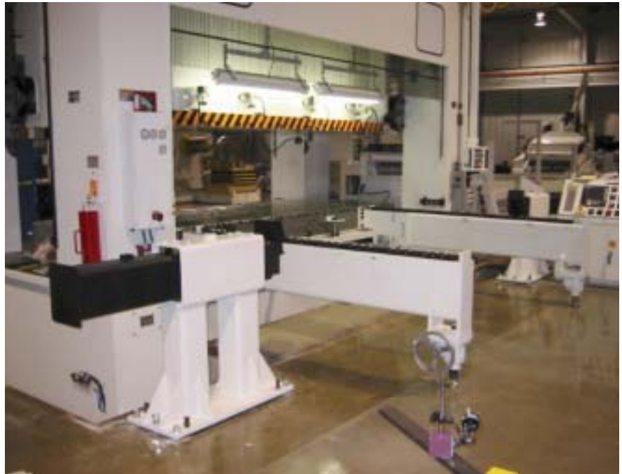
These 40,000-lb.-capacity pivoting bolster extensions allow for die loading by a forklift, and feature adjustable guides to accommodate multiple die sizes.
