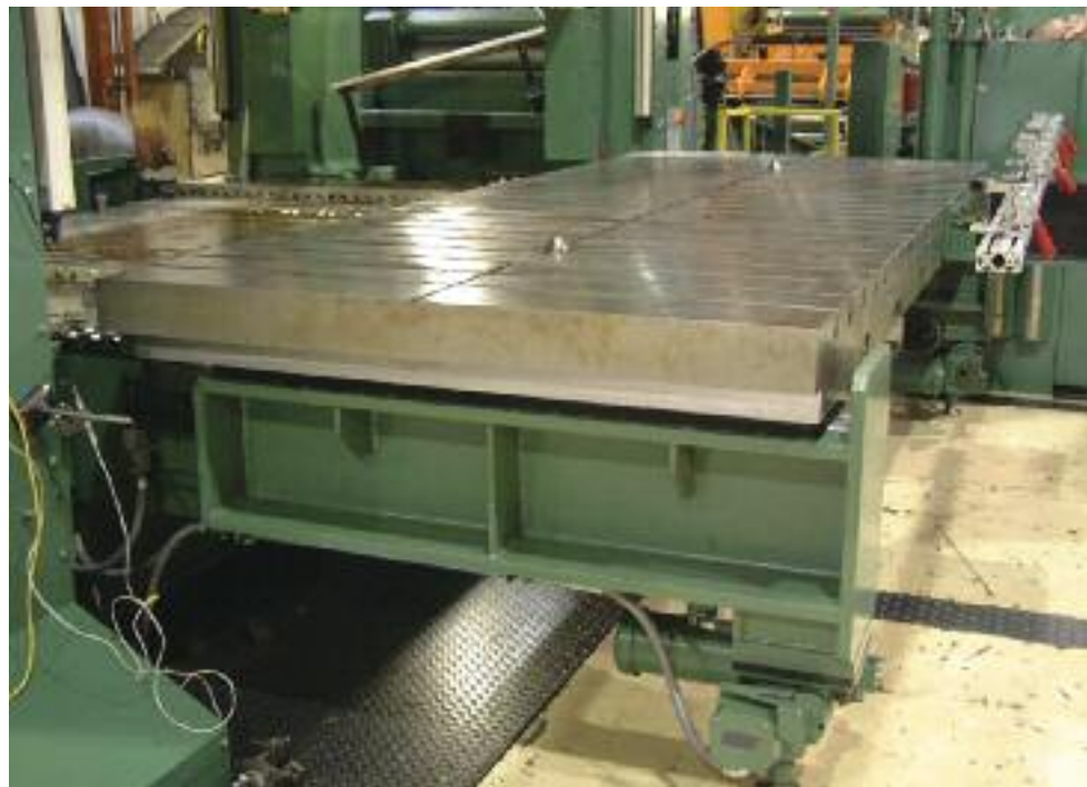
A raised rolling bolster retrofitted onto a press is an excellent method for optimizing die-exchange times.
